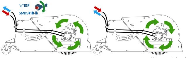
Motor mounted on right
