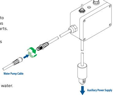
**WARNING:** Do not run the pump without adequate water.
