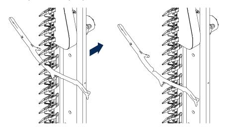
If branches become jammed in the trimmer keep the trimmer running and reverse away from the branch DO NOT change the cutting angle.
