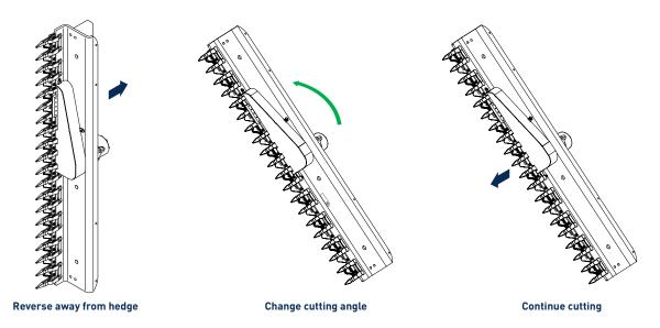
If branches become jammed in the trimmer keep the trimmer running and reverse away from the branch DO NOT change the cutting angle.
