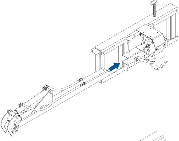
Push hitch bar (supplied with hedge trimmer) though the body assembly and fix using the rear hole position. The hitch bar can be fitted from either side always using the rear hole position.
