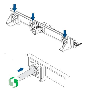
Once required position is located secure with fixing bolt and washers and tighten to 100Nm.
