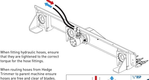
When routing hoses from Hedge Trimmer to parent machine ensure hoses are free and clear of blades.
