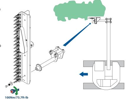
With the angle mount fitted between the double pin hitch and the hedge trimmer the cab and boom remain in line with the tracks.
