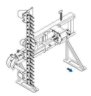
When both stands have been fitted and secured in position place the mount down on its stands and detach from parent machine.
