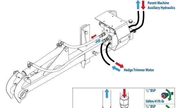
When fitting hydraulic hoses, ensure that they are tightened to the correct torque for the hose fittings.
