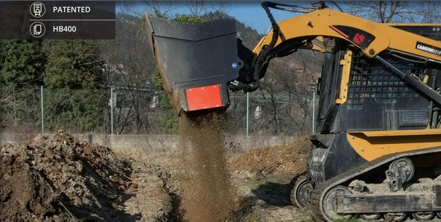
IT GRADES MATERIALS FROM DEMOLITION, DIGGING AND EARTH-MOVING WORKS. IT IS IDEAL ALSO FOR THE MIXING OF TERRAIN AND PEAT. THE CORE-ELEMENT IS AN HYDRAULIC SIEVE WITH ROTATING HB400 KNIVES. THE MATERIAL THICKNESS CAN VARY FROM 0 TO 20 (0 - 0,8 IN) AND FROM 0 TO 35 (0 - 1,4 IN) WITH A STANDARD EQUIPMENT.
